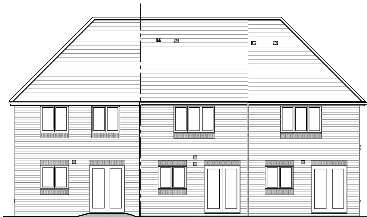
REAR ELEVATION 5P3B END (OPP)
