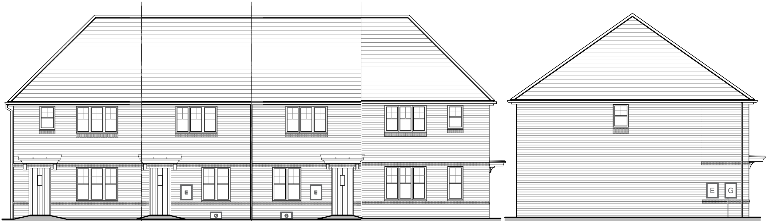
5P3B END (AS) FRONT ELEVATION 4P2B MID (AS) FRONT ELEVATION 4P2B MID (OPP) FRONT ELEVATION 5P3B CORNER (OPP) FRONT ELEVATION 5P3B END (AS) SIDE ELEVATION
