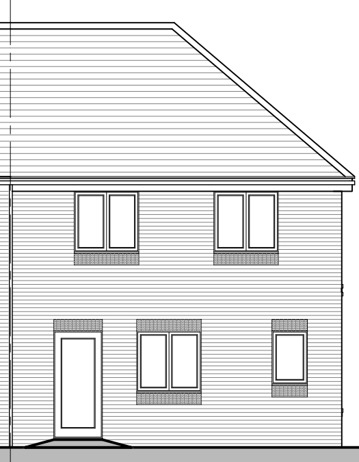
6P4B - FRONT GABLE (AS) REAR ELEVATION
