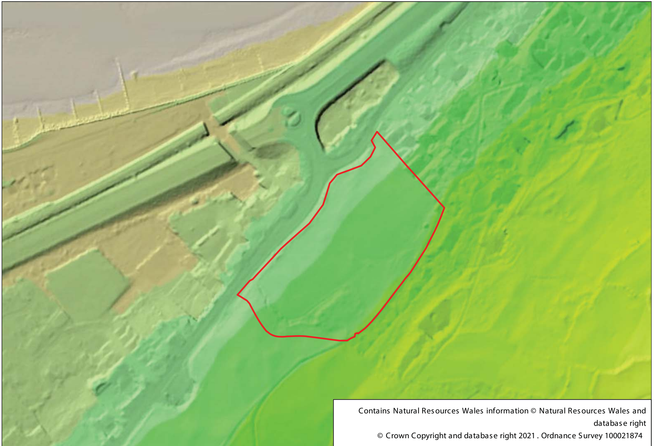
Figure 10: Reproduction of the Digital Light Detection and Ranging (LiDAR) 1m Digital Terrain Model for map sheet SH7860 (Source: Lle Geo Portal). Scale: 1:2500@A4
