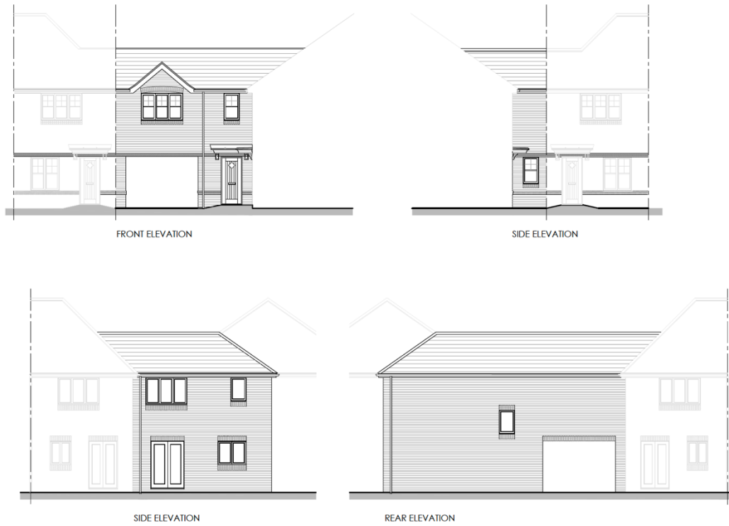
House Type: 4P2B Elevations
