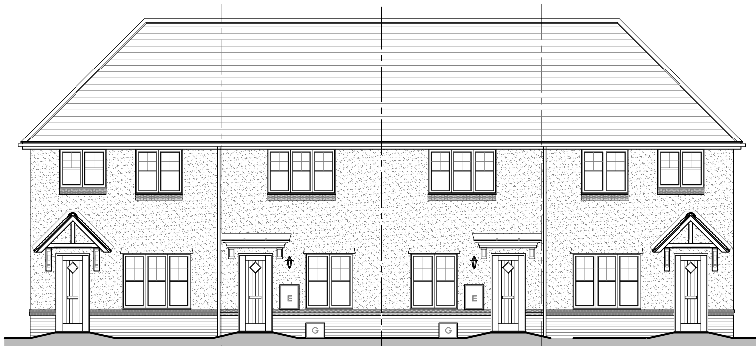
FRONT ELEVATION HR2 HIGHFIELD AS
