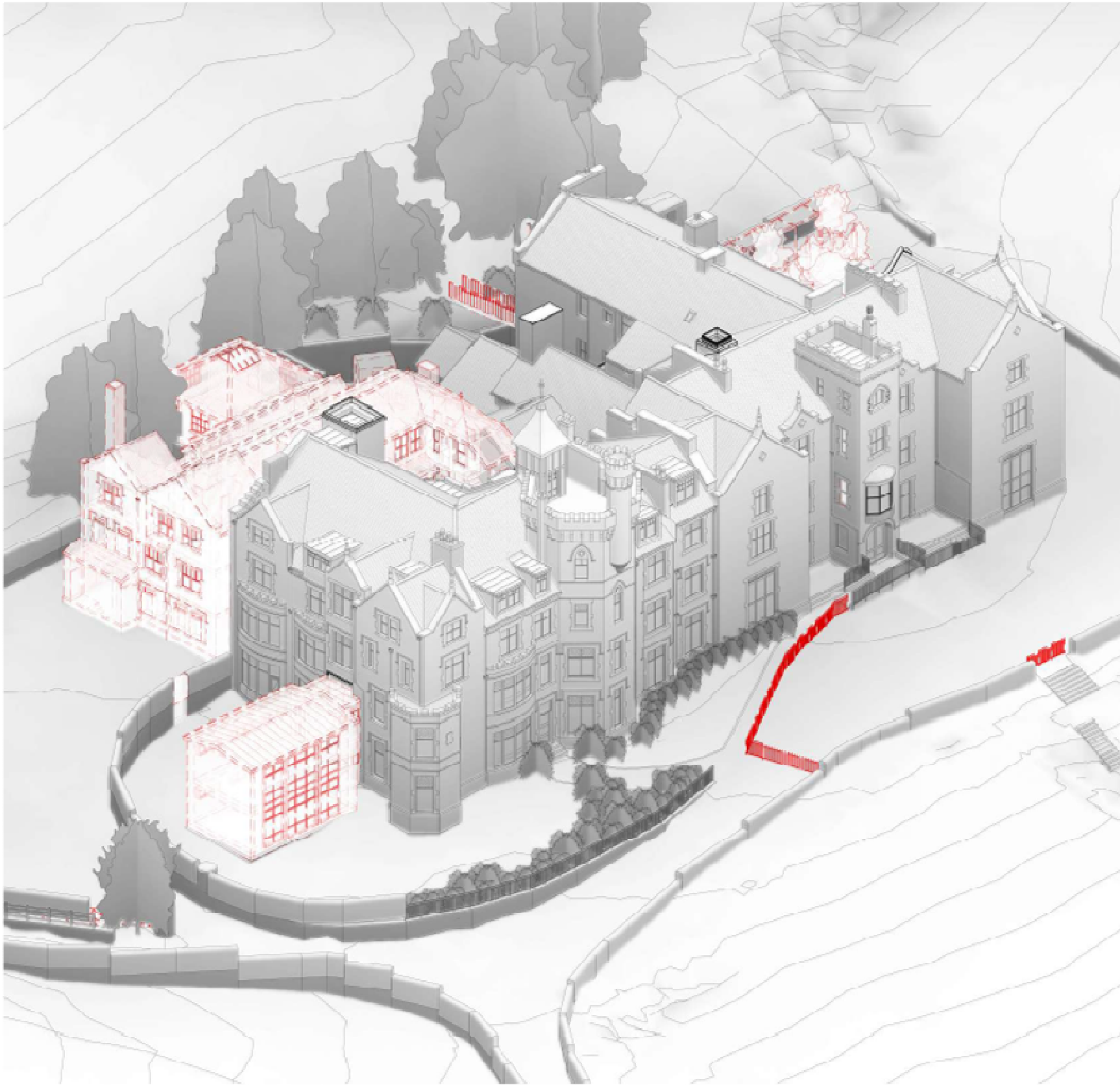
Image 01 - 3D East view of existing building showing parts to be demolished as modelled by AGa
